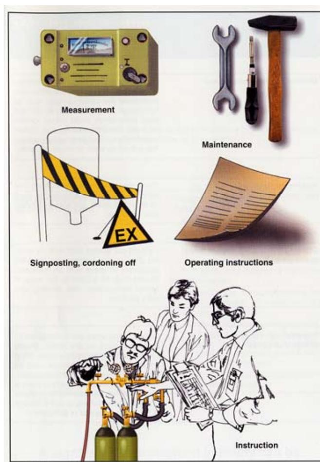
Figure 4.1: Examples of organisational explosion protection measures<sup>4</sup>
